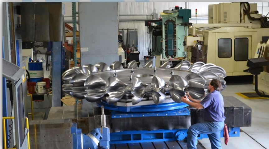
Figure 2: Final CNC machining of a stainless steel casting on Canyon's large 7-axis mill
