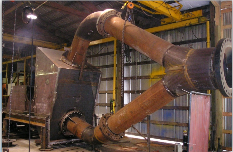
Figure 3: A572 steel housing and ANSI 300 Class water delivery system at Canyon's Deming facility
